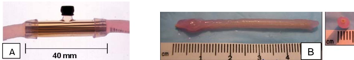
Figure 1. A: Hollow fiber bioreactor. The version shown has 6 longitudinal fibers. B: Development of cartilage from bovine chondrocytes after 4 weeks of growth.
